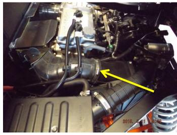
3. Separate the exhaust hose from the Clutch Housing.
