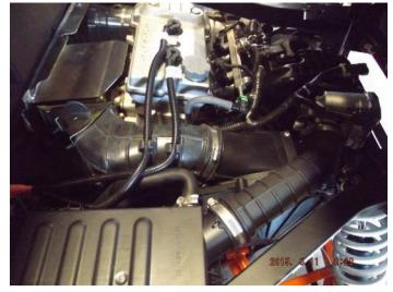
2. Loosen the clamp on the clutch exhaust hose.
