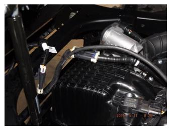
7. Plug in Blow Hole connector in line. The Blow Hole will run anytime the key is in the "On" position and for a brief 15 second time frame that the ECU keeps the chassis relay powered up after shutdown.
